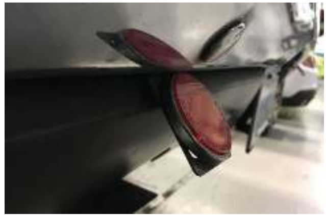
Two round reflectors, one per side, protrude beneath the rear bumper. These were a lighting regulation in Japan. Their presence is original and a cool talking point on this rare Japanese Mustang.
