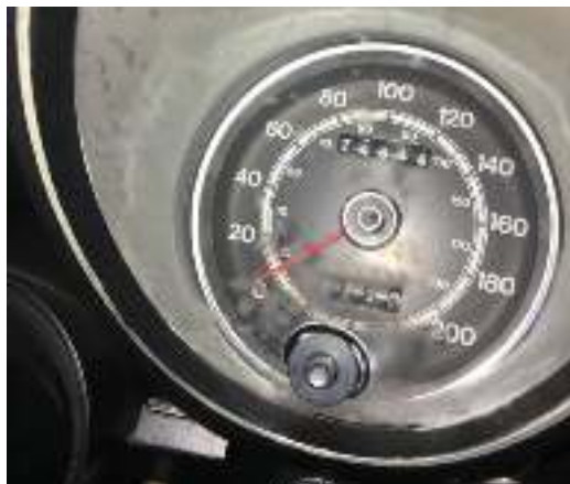
The odometer shows 79,646 kilometers, which is 49,490 miles. The speedometer for 1971 goes to 200 kilometers per hour (124 mph), while 1973s go to 220kph.
